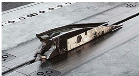
▲ CATAPULT SHUTTLE For catapult launches, a shuttle is attached to the plane's undercarriage and propelled along a short track by a steam-powered piston.
